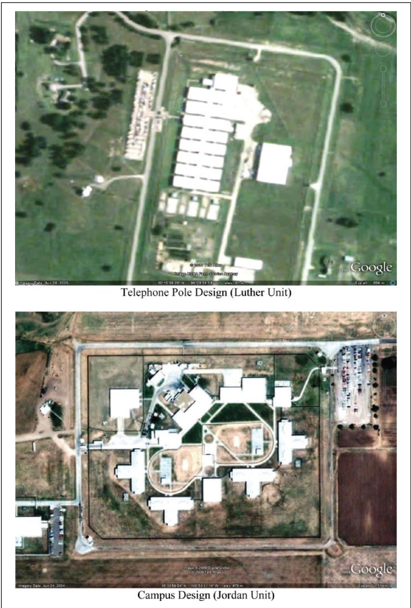
Figure 1. Prison architectural designs (aerial view): (A) Telephone pole design (Luther unit); (B) Campus design (Jordan unit).
